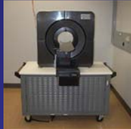
microPET P4 scanner PET resolution ~ 2.5 mm
