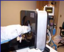
ImTek SPECT/CT scanner SPECT resolution ~ 1.5 mm CT resolution ~ 0.05 mm
